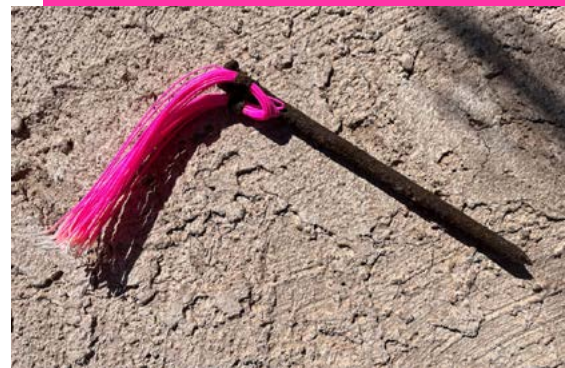
This is a property peg, one of many used to mark lot lines and the location of walls within Solera
